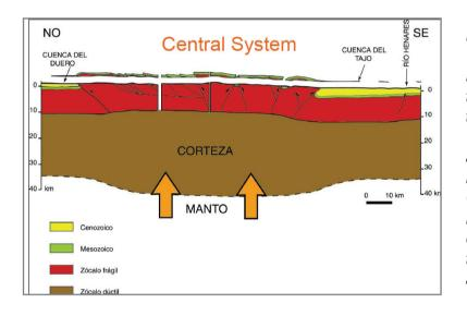
**Fig. 13:** The Central System: The compression of the Iberian block in Miocene times led to the deformation, folding and thickening of the crust itself (crustal, or lithospheric folds) and to the uplifting of big granite blocks, to form the so-called Central System. In the margins, both N and S, the Mesozoic cover was deformed and Tertiary continental basins (Duero and Tagus) were developed.
