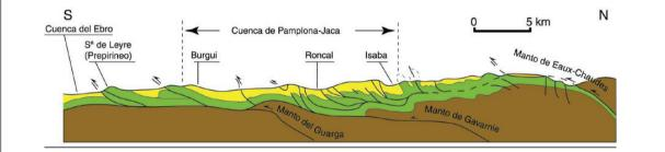
**Fig. 10:** The Pyrenean orogene: In Surface, the Mesozoic and tertiary cover, pushed by the crust thrusting has moved southwards forming large nappes and sliding on detachment levels, normally on the clay intervals of the Upper Triassic.
