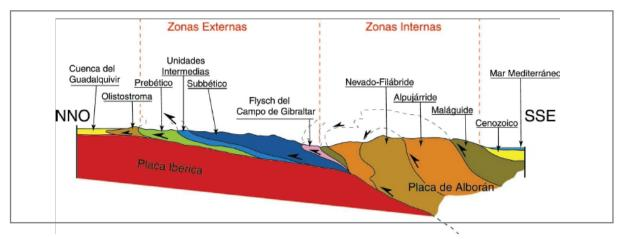
**Fig. 12:** Baetic orogene: The violent compression of African plate against Iberia in Miocene times from SE to NW led to the thrusting and piling up of many external and distant orogenic units on the southern margin of Iberia, and the subduction of this part of the Iberian bock. The piling up of nappes to the north led to the sinking of Iberian plate and the development of the tertiary basin (Foreland basin) of Guadalquivir.
